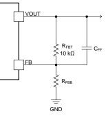
Figure 17. Setting the Output Voltage
