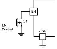
Figure 22. Typical Enable Control
