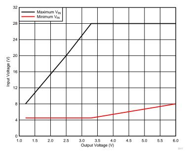
Figure 18. Input Voltage vs Output Voltage
